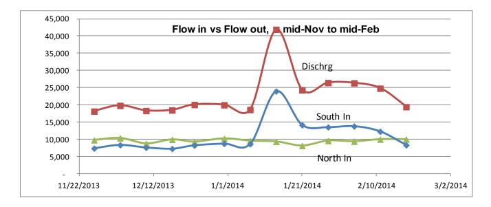
[We now know the most likely increase in southside inflow was due to a broken water pipe at a residence on South LSD. We learned about the broken pipe in Feb from C. Holland. We also learned that the broken pipe was discovered (and flow stopped) on Feb 8. -- RH]
