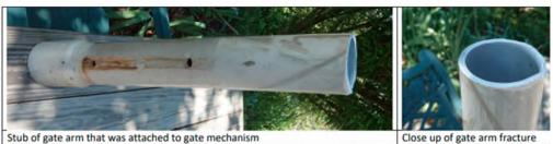
Janet & I put on new gate arm at about 7:30pm June 13. Outgate arm broke due to fatigue over a period of a few hours (or years of use!). Gate was NOT sawed off, though it looked like it. Break was so clean it looked like it had been sawed. Normally when a gate arm breaks from fatigue, it breaks at a drill hole. Not this time.
